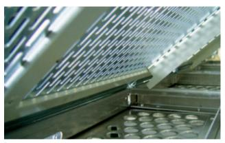
Screensegment within exchangeable screen frame
